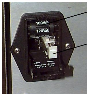
**Figure 3.3 Power Entry Module**
