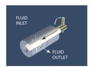
POSITIVE DISPLACEMENT IS CREATED DURING THE DISCHARGE STROKE AS THE PISTON ADVANCES INSIDE THE CYLINDER. THE PISTON FLAT OPENS THE OUTLET PORT TO THE PUMP CHAMBER AND THE INLET PORT IS CLOSED.
