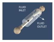
IN THE DISCHARGE STROKE POSITIVE DISPLACEMENT IS CREATED BY THE LINEAR MOTION OF THE PISTON.
