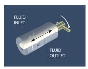
THE PISTON IS SHOWN AT BOTTOM DEAD CENTER OF ITS STROKE. BOTH INLET AND OUTLET PORTS ARE CLOSED AND PISTON FLAT IS ROTATING TOWARD THE INLET PORT.
