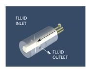
POSITIVE DISPLACEMENT IS CREATED DURING THE DISCHARGE STROKE BY LINEAR MOTION OF THE PISTON.
