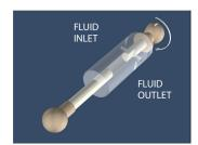
THE VALVE ROTATES 180° AND THE FLAT OPENS THE OUTLET PORT TO THE PUMP CHAMBER – THE INLET PORT IS CLOSED.
