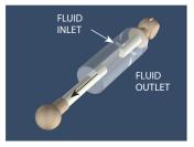
SUCTION IS CREATED DURING THE INTAKE STROKE BY THE LINEAR MOTION OF THE PISTON.
