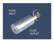
The piston rotates 180° and the flat on the piston opens the outlet port to the pump chamber – the inlet port is closed.
