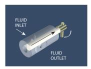
SUCTION IS CREATED DURING THE INTAKE STROKE BY THE PISTON RETRACTING INSIDE THE CYLINDER. THE PISTON FLAT OPENS THE INLET PORT TO THE PUMP CHAMBER AND THE OUTLET PORT IS CLOSED.
