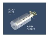
THE PISTON IS SHOWN AT TOP DEAD CENTER OF ITS STROKE. BOTH THE INLET AND OUTLET PORTS ARE CLOSED AND PISTON FLAT IS ROTATING TOWARD THE OUTLET PORT.
