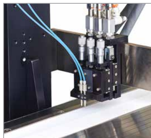
Dispensing 2 Reagent Lines onto Substrate
